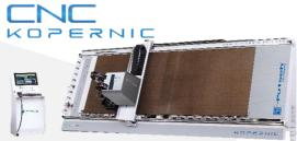
The Putsch® CNC Kopernic Vertical Machining Center is the right CNC which allows to process various kinds of panels while saving space in the work room.
