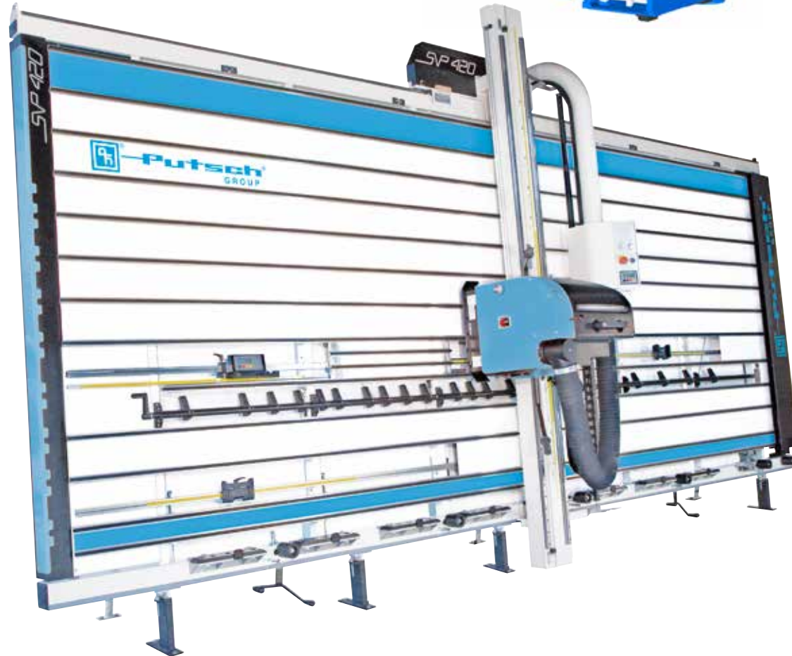
The newly developed “Posi-System” automatically positions the vertical stop for cross-cuts and the saw head for horizontal rip cuts.
