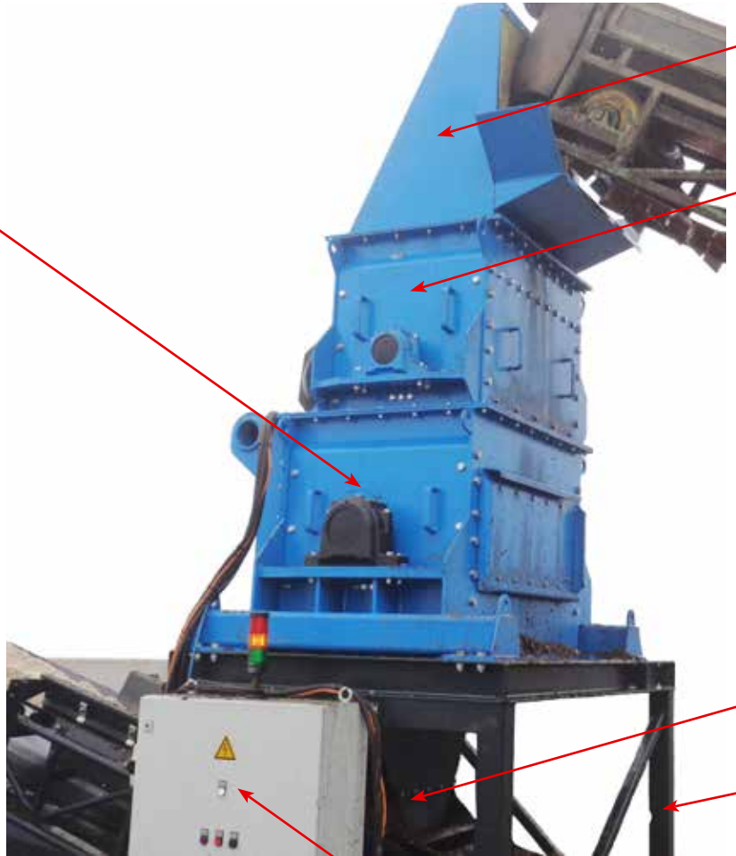
Electrical Cabinet with overload indicator
