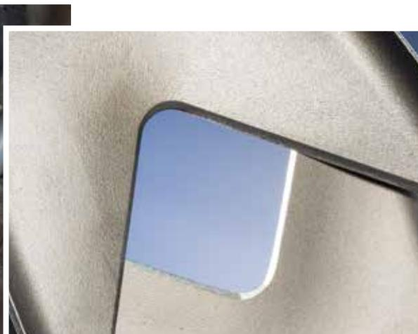
**The precise grinding of the cutting edges ensures an exact separation of the glass flow and the uniform drop of the glass gob in the machine. /**
