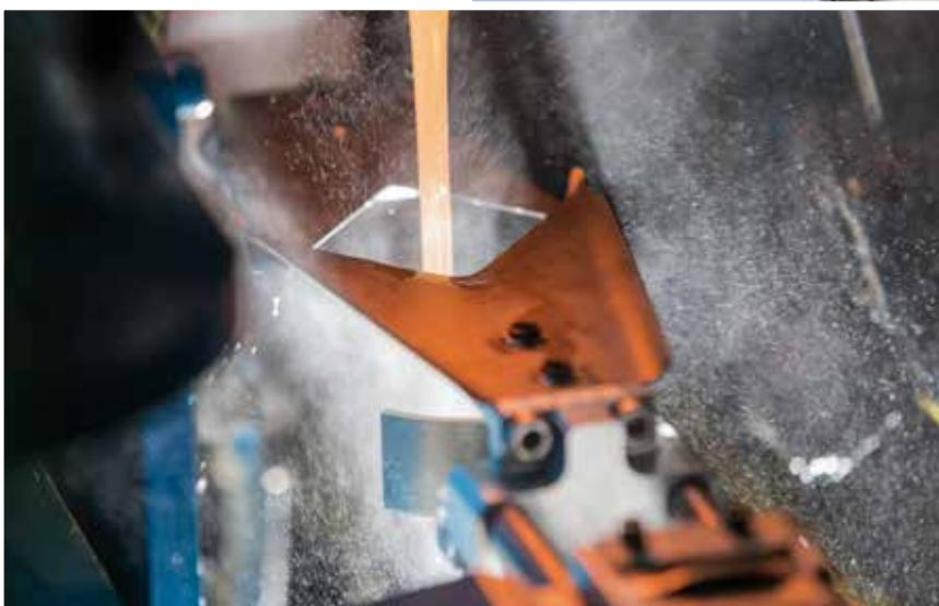
*Due to the high level of parallelism and flatness of Putsch® shear blades, the difference between the individual blades can easily be fine-tuned and the cutting edge pressure is reduced to a minimum. /*
