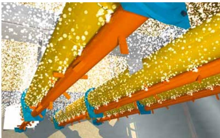
*The fine CO<sub>2</sub> bubbles leave the Putsch® Richter Tubes through the precisely dimensioned slots facing the vessel bottom.*
